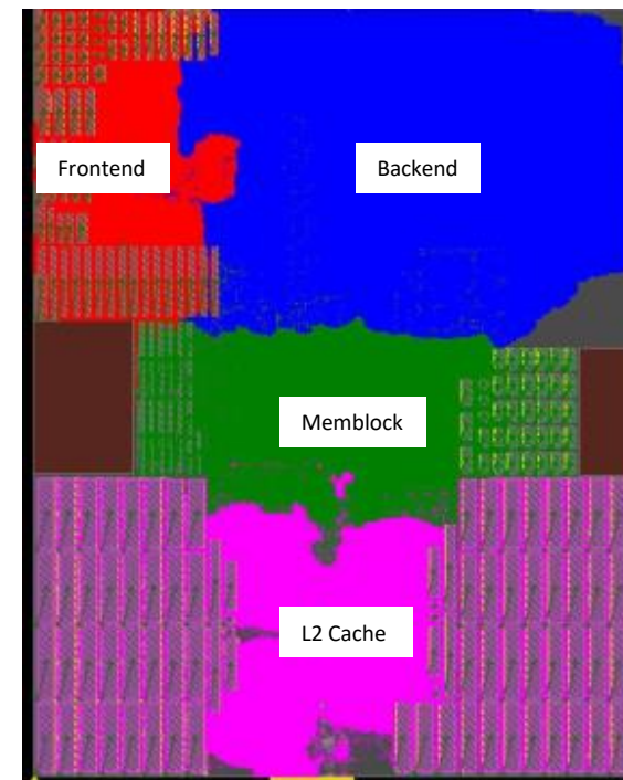
Floorplan of V1 (single core)
